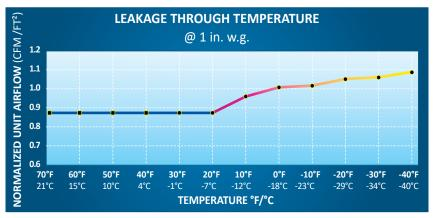
Damper tests were conducted in a laboratory cold room to determine the effects of colder and severe cold temperatures (down to  $-40^{\circ}F(-40^{\circ}C)$ ) on sealing gaskets and leakage rates.
